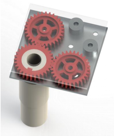
Figure 4.1 Singularity's new turn sensor gear train
